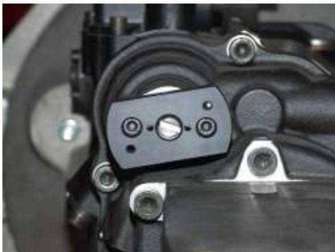
This photograph shows the adapter in position on an SCL82-14 with the gearbox in neutral.
