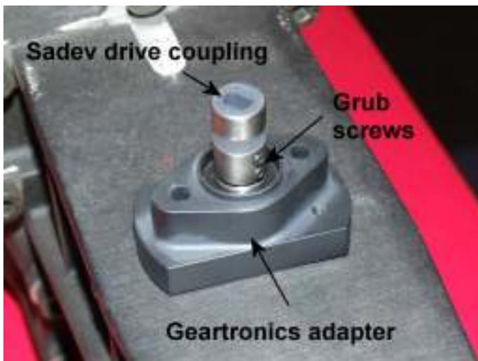
When using a Geartronics sensor adapter with a Sadev gearbox, it's very important to position the Sadev drive coupling so that reverse (red) and 6<sup>th</sup> (pink) gears are either side of the 0° position as shown above. Some trial and error will be required to position the sensor correctly, but the easiest method is to select 3<sup>rd</sup> gear, then rotate the sensor by hand to the 180° position (dot pointing at cable) before securing the drive coupling with the two grub screws.
