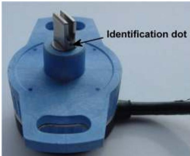
When this dot is pointing directly opposite the cable, the sensor is positioned in the dead band. Conversely, when the dot is aligned with the cable, the sensor is mid-travel and the output voltage will be 2.5v.
