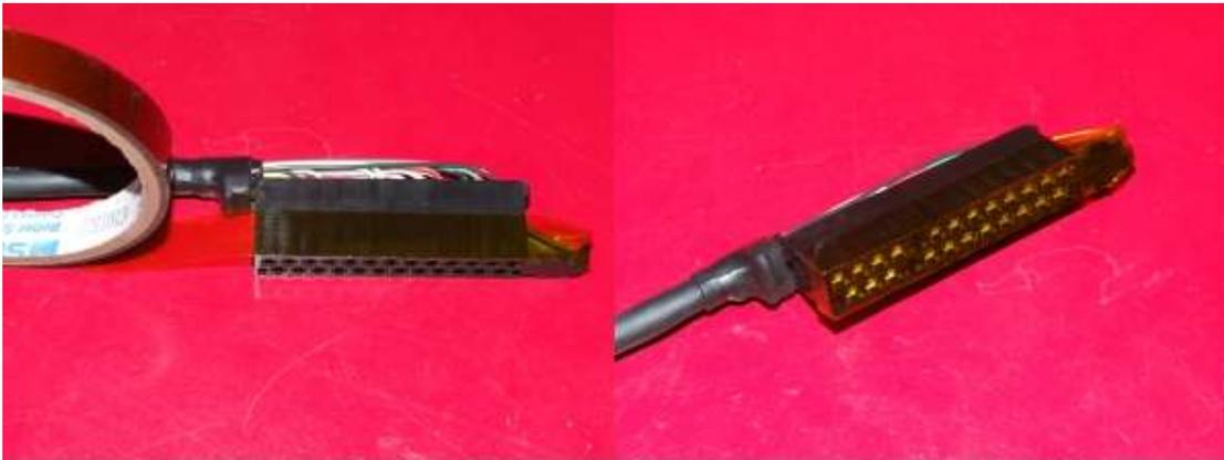
In order to seal the rear of the connector and improve the mechanical reliability & aesthetics, a large piece of adhesive-lined sleeving is applied over the entire connector housing. This sleeving must have a shrink ratio of 4:1 to that it will shrink down sufficiently to seal the cable exit.
