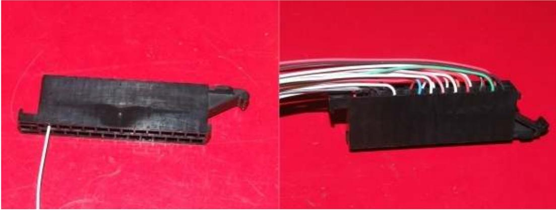
Next, place the connector in a vice and temporarily secure the wires to the housing using a cable-tie as shown below. Carefully twist the wires in a uniform pattern up to the first harness transition. Twisting the wires adds greatly to the flexibility of the harness, and also helps with noise immunity. Experienced harness constructors may employ a contra-helical twist pattern for even greater flexibility & reliability.
