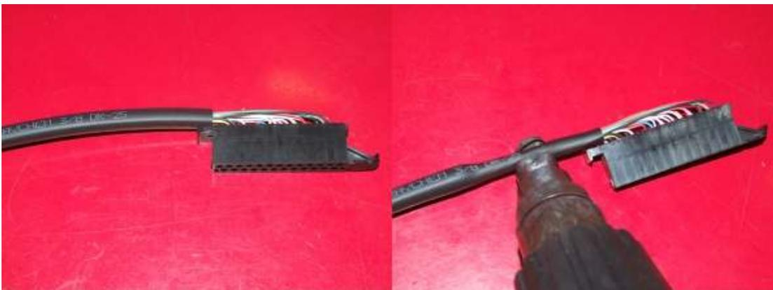
Next, place a Raychem moulded boot, part #: 202A111, over the wires. Make sure the thickest end is closest to the connector housing. For increased reliability, 'RT125' 2-part glue should be used on the inside of the boot. Gently shrink the boot, being careful to initially direct the hot air closer to the thick end of the boot in order to prevent the thin end folding back on itself!
