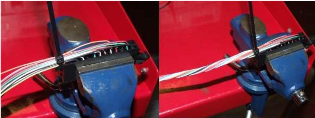
When you are satisfied that the wires are twisted correctly, cover with the appropriate size of DR25 sleeving. Push the sleeve as far as it will go over the bundle of wires. Most GCU harnesses with approximately 20-23 conductors will require 3/8" diameter (un-shrunk) sleeving. Using the correct wiring heat gun (not a paint stripper!) gently shrink the sleeving down onto the wires, taking care not to overheat the sleeve or melt the connector.
