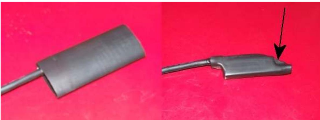
When you have fully shrunk down the sleeving, use a pair of pointed-nosed pliers to seal the end as shown by the arrow in the above picture.
