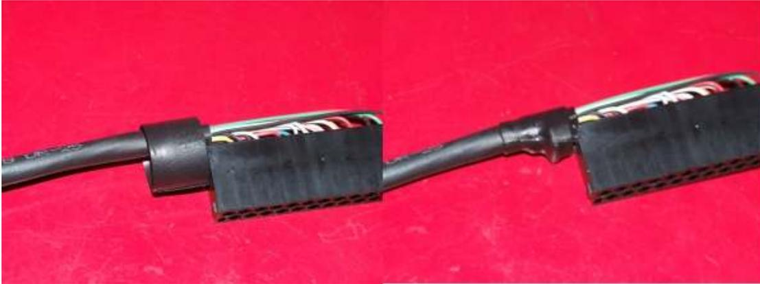
The next job is to apply Kapton tape to the lower half of the connector. When the adhesive-lined heat-shrink tube is applied in the next stage, the tape provides a mask to prevent glue entering the contacts.
