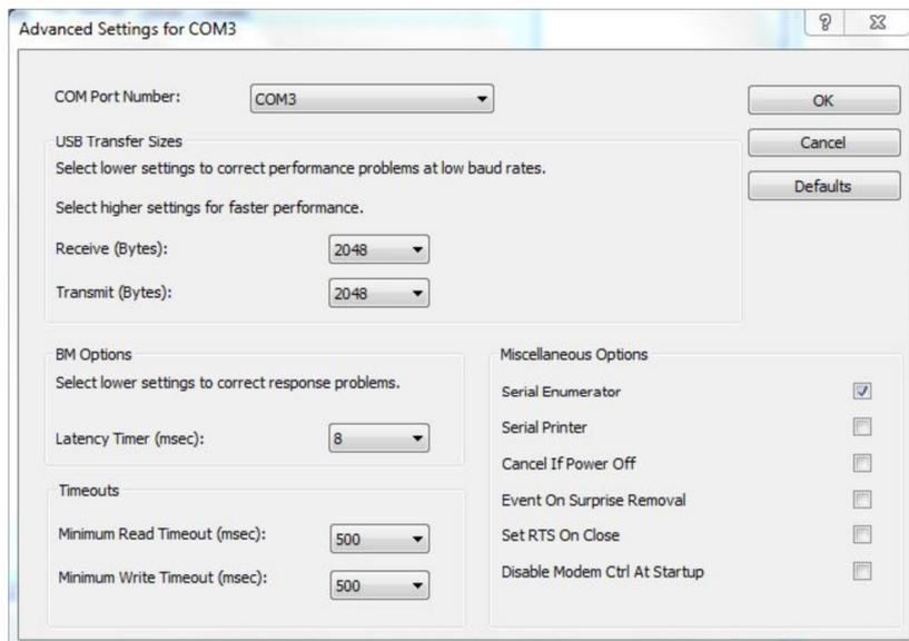
These settings relate to the on-board FTDI driver chip in the GCU, but external Prolific chips have similar properties. The latest Geartronics driver already has the above properties configured by default.
